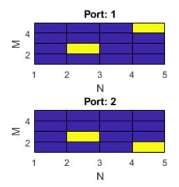
Create a 3D received grid to extract resource elements. Extract resource elements from the received grid. Show the locations of these extracted resource elements. Addressed resource element locations contain 1.
