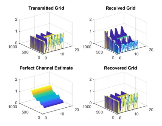
Comparing the transmitted grid to the recovered grid shows equalization of the received grid with the perfect channel estimate recovers the transmission.
