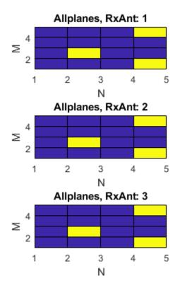
Create a 4D channel estimate grid to extract resource elements. Extract resource elements from the channel estimate grid. Show the locations of these extracted resource elements. Addressed resource element locations contain 1.
