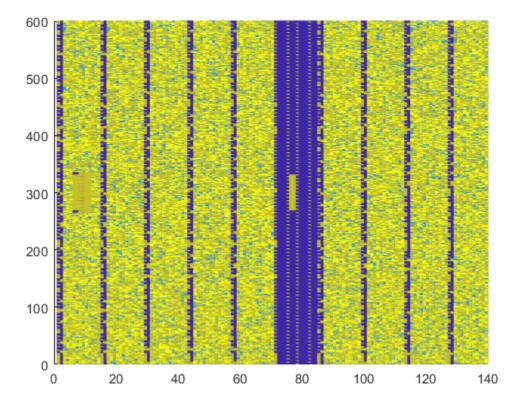
To insert SIB1 message into the output waveform, initialize SIB substructure, enable SIB transmission, adjust other defaults, and regenerate txGrid. Plot txGrid to illustrate the presence of SIB1 message in subframe 5
