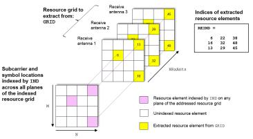
The following diagram shows the extraction process for a 4D channel estimate grid, grid, with NRxAnts = 3 and P= 2. In this case, P is the number for antenna ports. The 4D resource grid consists of P M-by-N-by-NRxAnts arrays, each associated with an antenna port. Resource elements are extracted from all planes within these arrays.
