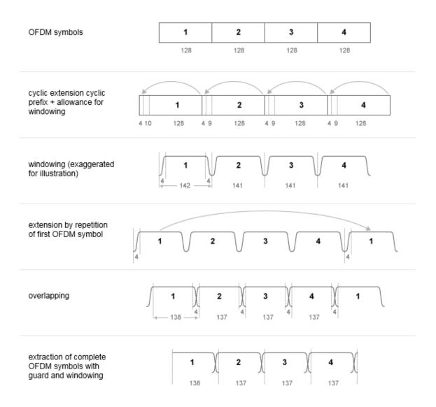
The number of samples used for windowing depends on the number of resource blocks and whether the cyclic prefix length is normal or extended. The number of samples is chosen in accordance with the *maximum* values implied by TS 36.101 [1], Tables F.5.3-1, and F.5.4-1.
