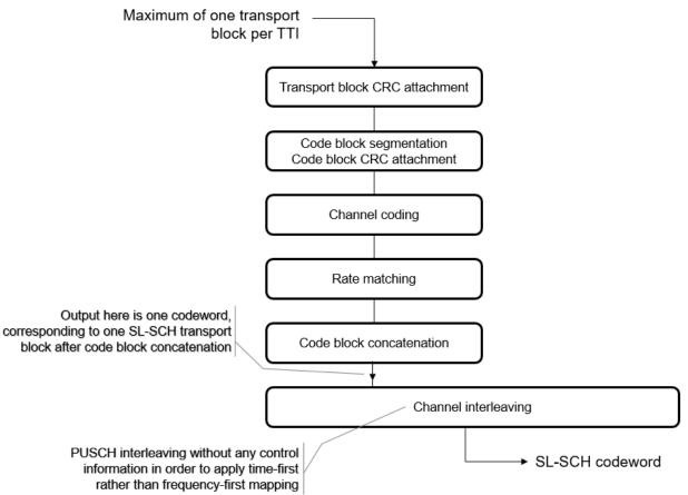
The SL-SCH transport channel codeword carrying the information bits of a single transport block is transmitted on the physical sidelink shared channel. Use the ltePSSCH and ltePSSCHIndices functions to generate the modulated symbols and populate the resource grid for transmission.
